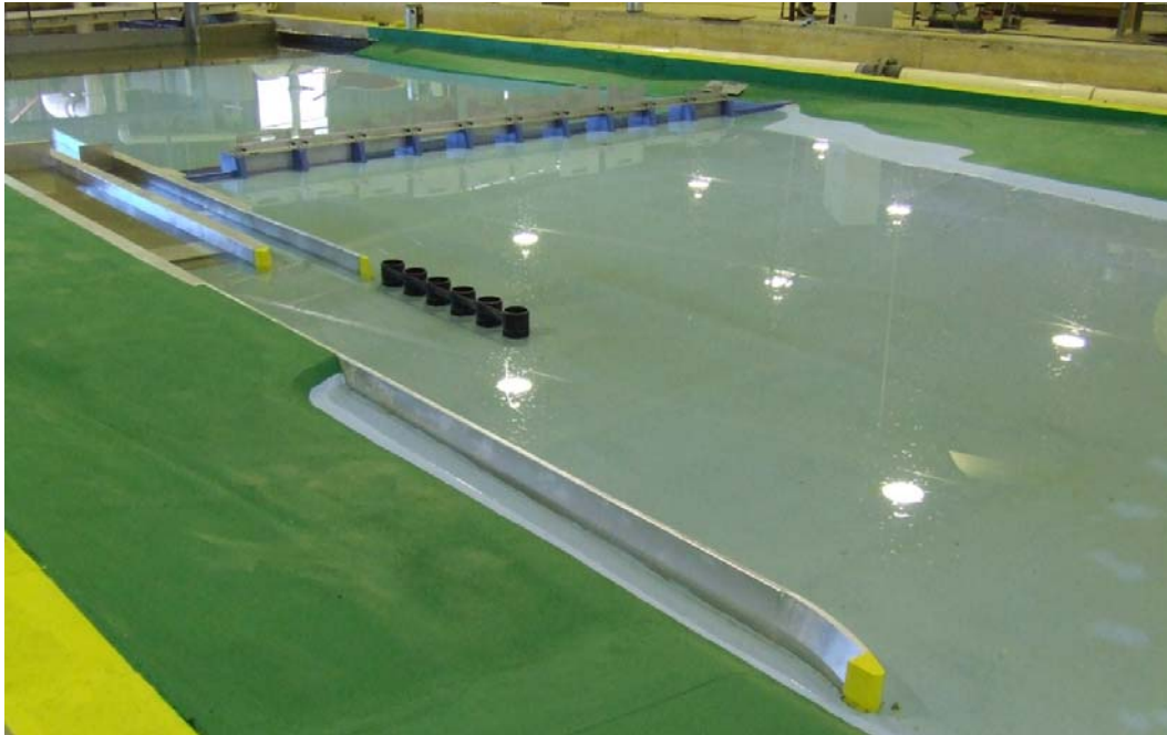
Figure 5. Photograph of physical model looking downstream, Plan A lock approach.
