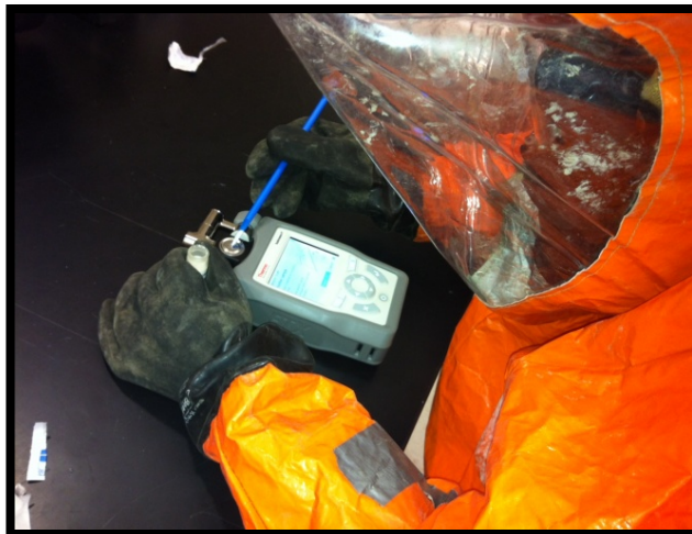
Figure 8: Processing a Sample in Level A PPE
