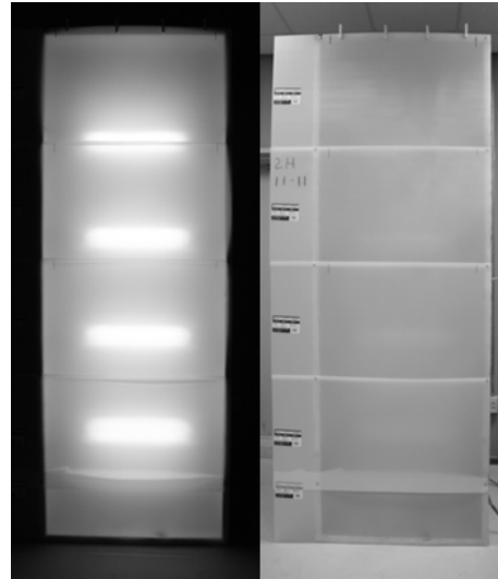
Figure 6. Light Box during Operation (left); Light Box Shown in Daylight Showing 4 ½ Sheets of Commercially Available Light Diffusers (right)
