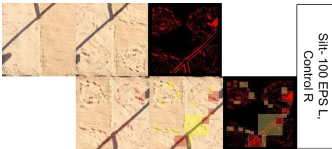
Figure 21. large scale testing utilizing both the EPS material at 100 kg/acre and the a water control in the same test plot (EPS on the left, control on the right). Four objects were implanted in each treatment area and the automated detection system attempted to identify the implanted areas automatically.
