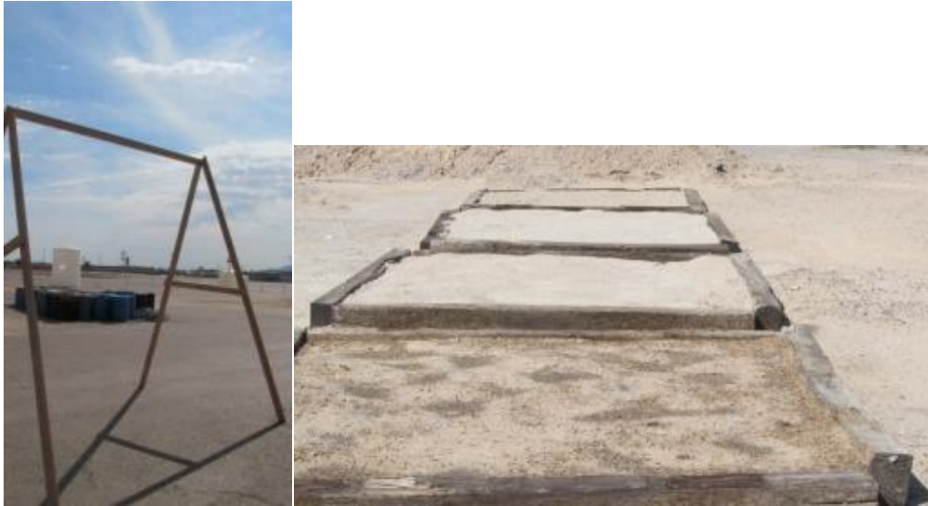
Figure 14. Frame used to support aerial camera used to take photos of un-tampered and tampered soil plots. The size of the implanted or disturbed area could be modified to simulate detection at locations from 1 foot to 200 ft above the ground, depending on the implanted object size and distance of the A frame from the plots
