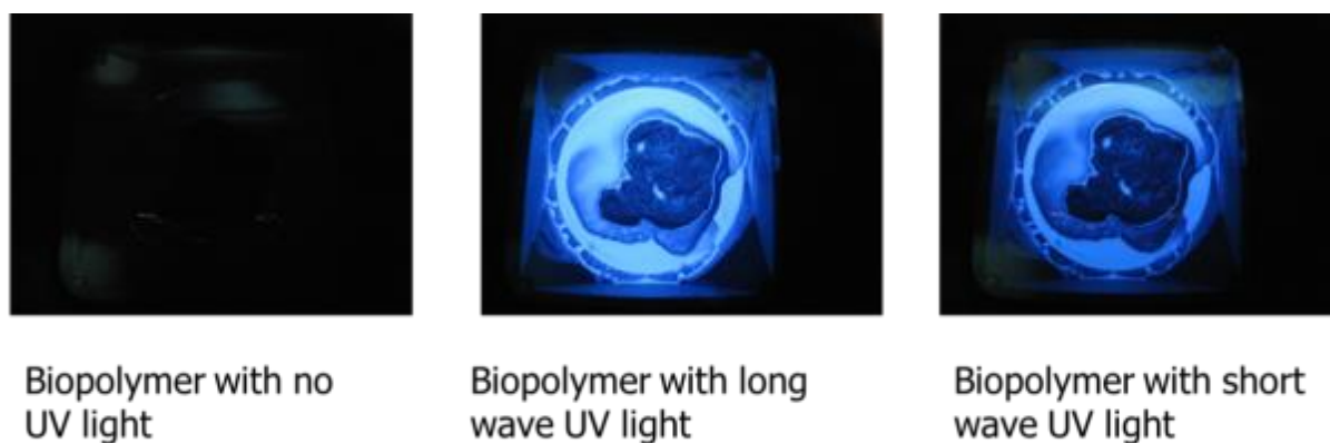
Figure 29- Alternative tagged EPS synthesis where a fluorophore was mixed into a microbial mixture to determine if the microbes would incorporate the tags into the biopolymer.
