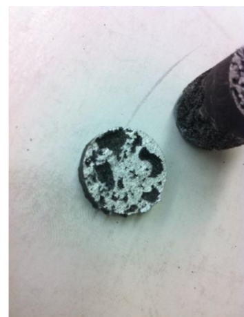
Figure 2: Tungsten powder in aluminum in a casting furnace at 950 C.
