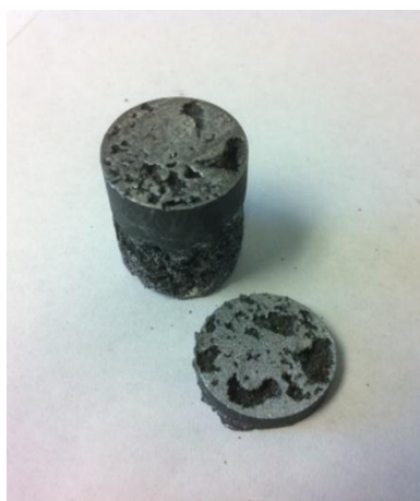
Figure 2: Tungsten powder in aluminum in a casting furnace at 950 C.
