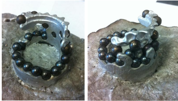
Figure 6: Stainless steel sphere casting results. Pouring at 790 °C. Standard annular sand casting mold.
