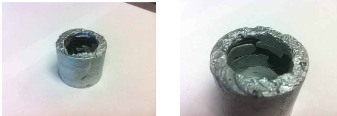
Figure 7: 0.010" diameter tungsten wire cast. Preheated mold and tungsten wires before pouring at 790 C.
