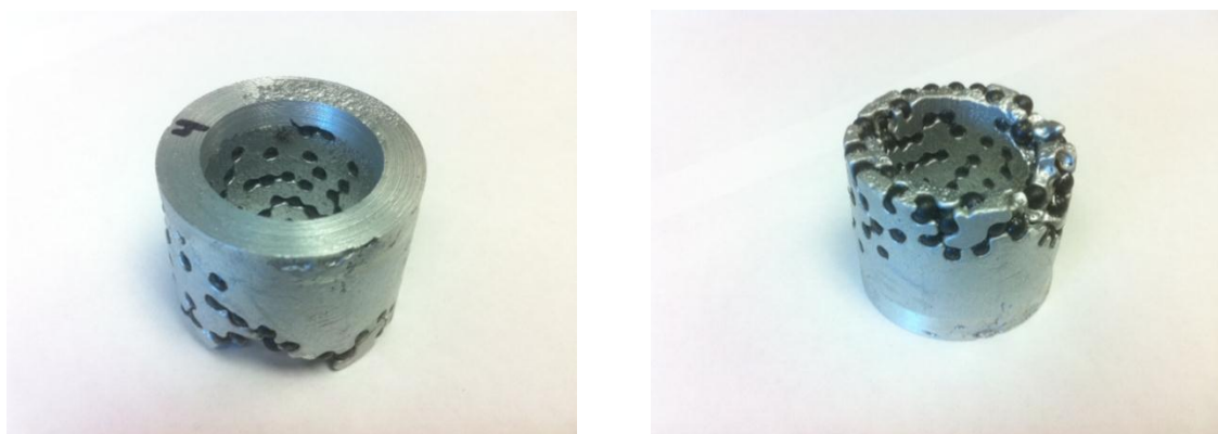
Figure 9: 4 mm diameter tungsten sphere cast. Preheated mold and tungsten spheres before pouring at 790 C.
