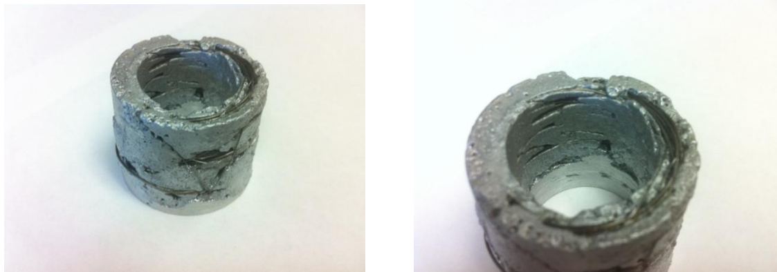
Figure 8: 0.025" diameter tungsten wire cast. Preheated mold and tungsten wires before pouring at 790 C.
