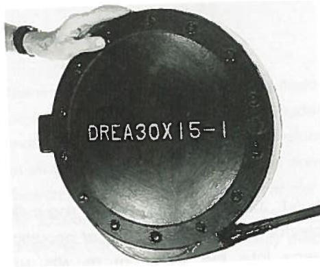
Figure 3.1: The depth-compensated ring shell projector [2]
