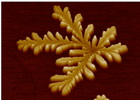
Figure 85. An atomic force microscope image of a self-assembly electrical circuit. The diameter of the circuit is 5 microns.
