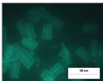
Figure 87a. Epi-fluorescent microscopy of FITC-labeled PLL adsorbed on diatom thin film.
