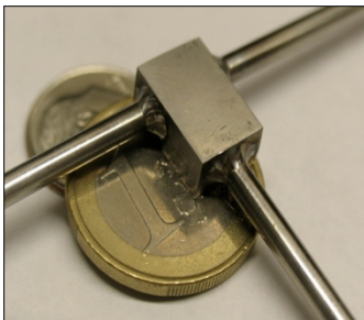
Figure 62. Picture of a SS micromixer produced by diffusion bonding of thin laminae and micro-welding of inlet and outlet tubing.
