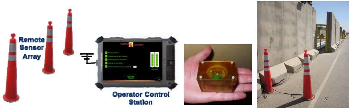
Figure 2. Left-to-Right: The SubtleMadness unattended ground sensor security system - sensors are obscured under traffic cones and laid out in an array depending on the protection scenario; The Operator Control Station tablet PC can be located up to 1000 meters from the sensor array providing safe standoff and automated alarm indications; A miniaturized magnetic sensor in the palm of the hand; The SubtleMadness physical security system protecting an entry control point in central Iraq.
