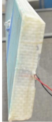
Figure 3: Side view of the Beam showing the sensor wires
