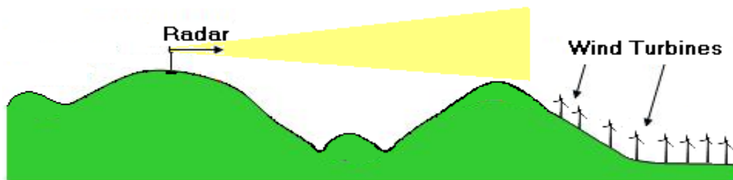
Figure 38. This illustration shows the use of terrain masking as one way to mitigate the impact of wind turbines near a radar site.
