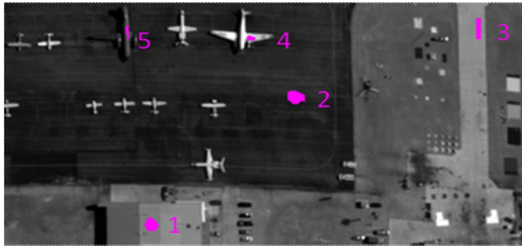
Figure 10. Example frame of one band of hyperspectral data from ASIP sensor. The five classes of interest are: #1: metal roof; #2: tarmac; #3: concrete; #4: white plane; #5: blue plane.
