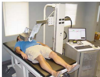
Fig. 1. Mobile gantry system in a bedside environment with the detector head in an anterior position for acquisitions in the single photon detection (SPECT) mode.
