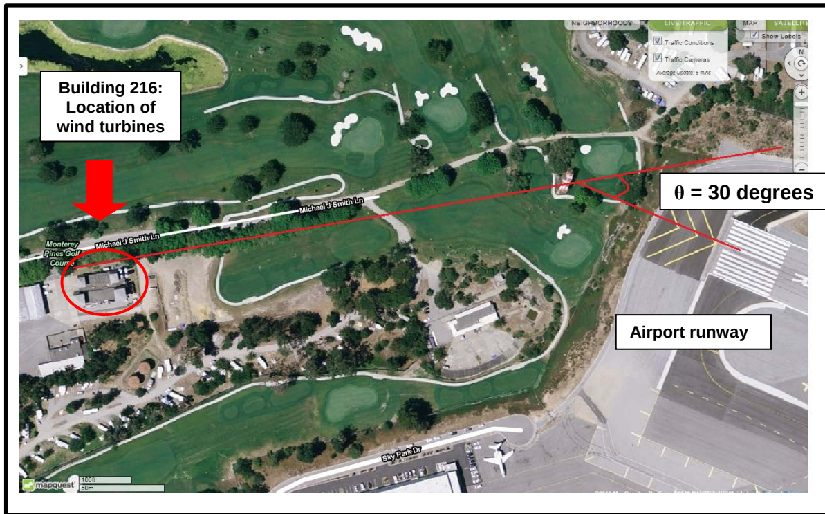
Figure 7. Orientation of the Monterey Airport runway in relation to Building 216. After [10].
