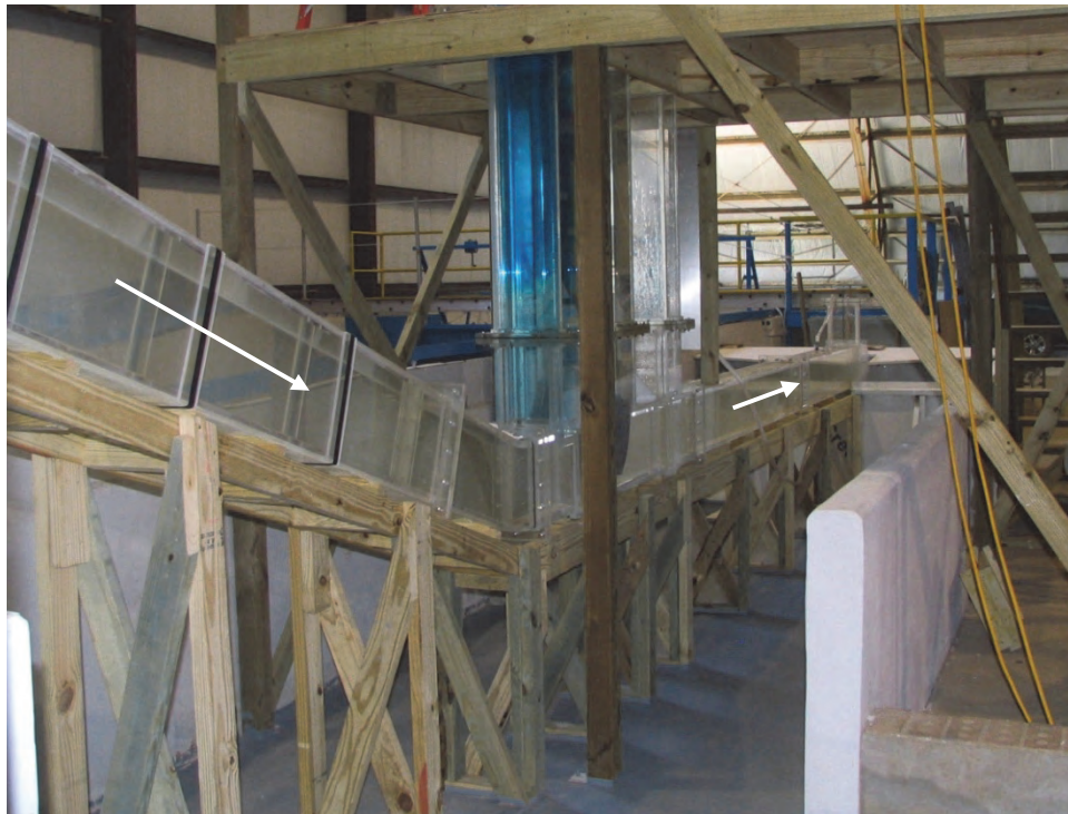
Figure 8. Lock Culvert Model – Downstream View
