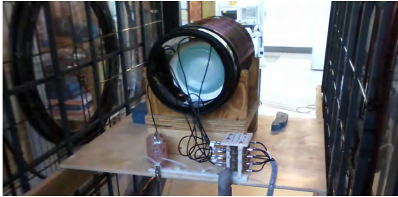
Figure 25: Test setup of 8 channel parallel imaging coil and phantom inside a 25 cm transmit coil in the 6.5 mT electromagnet LFI. The pale blue color is the CuSO 4 -doped water phantom.
