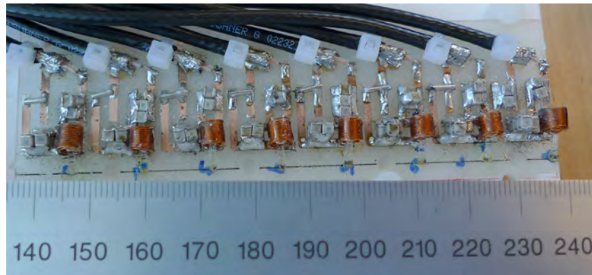
Figure 9: Array of 8 miniature NMR field probes spaced at regular intervals along a positioning arm. The arm is mounted on a fixed cylinder that is concentric with the bore of the Halbach magnet. The magnet is rotated around the field probes, allowing the frequency to be measured at different points within the bore. The arm can also be translated along z to acquire additional slices for the field map. Ruler marks are mm. Water bulbs are 3 mm.
