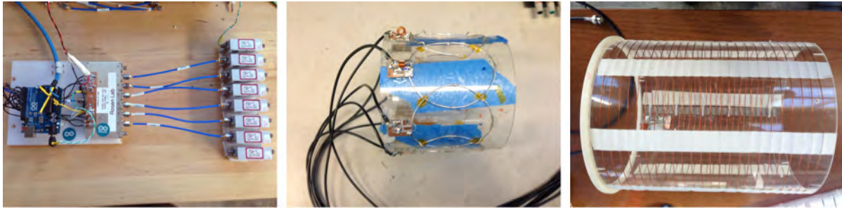
Figure 17: RF subsystem includes ( left ) multiplexing 8-to-1 switch with a bank of 8 pre-amplifiers, ( center ) 8-channel array of receiver loops, and ( right ) solenoid transmit coil for producing a uniform B_1 field.
