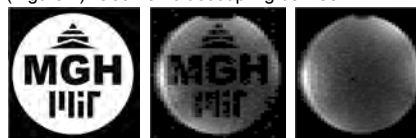
Figure 2. Phantom pattern (A), reconstruction of structured phantom (NA=150, B) and reconstruction of homogeneous phantom (NA=200, C). Images are masked to the phantom.
