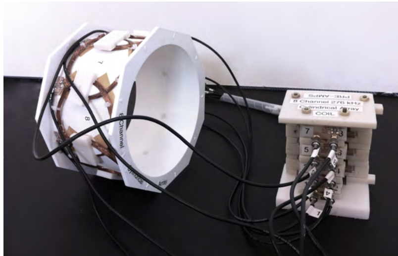
Figure 24: The final eight-channel array coil ( left ) and the tune/match electronics stack ( right ).
