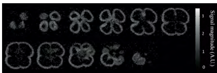
Figure 1: 11 slices of the imaged bell pepper at 6.5 mT with 2.7×2.5×9 mm 3 resolution in 12.6 min.
