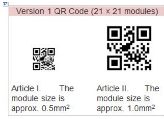
Figure 15. Setting the module size (From Denso-Wave, 2012)
