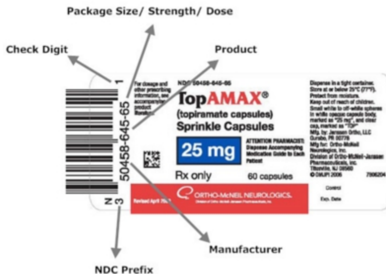
Figure 23. Deciphering NDC Barcodes (From RX Scan, 2013)
