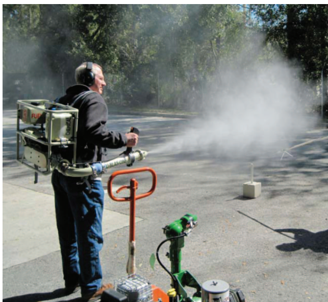
Fig. 7. Prototype ULV backpack sprayer (U-BLAS-ONE) built by DAT and evaluated during annual “equipment rodeo” conducted by the Navy Entomology Center for Excellence (NECE). Photo: Todd Walker.
