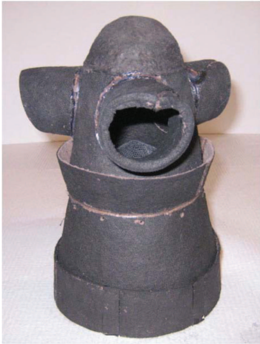
Fig. 3. Prototype pyriproxifen autodissemination station for use against Ae. aegypti and Ae. albopictus . Photo: Randy Gaugler.
