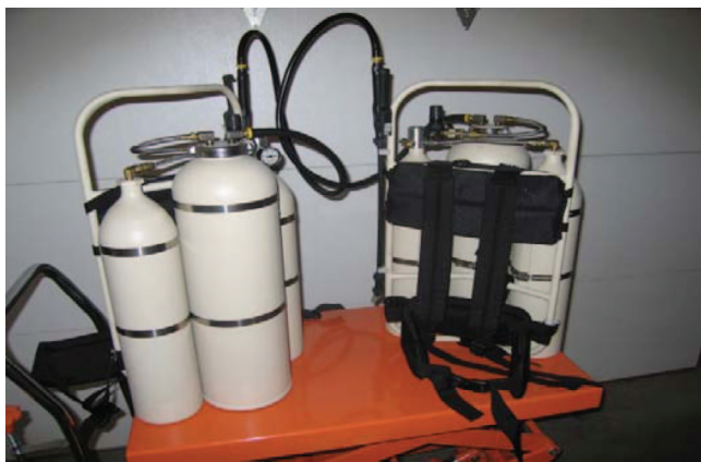
Fig. 6. Compressed air-powered backpack sprayer (JQX) that silently delivers a constant flow rate and consistent droplet spectra. Photo: Bruce Dorendorf.
