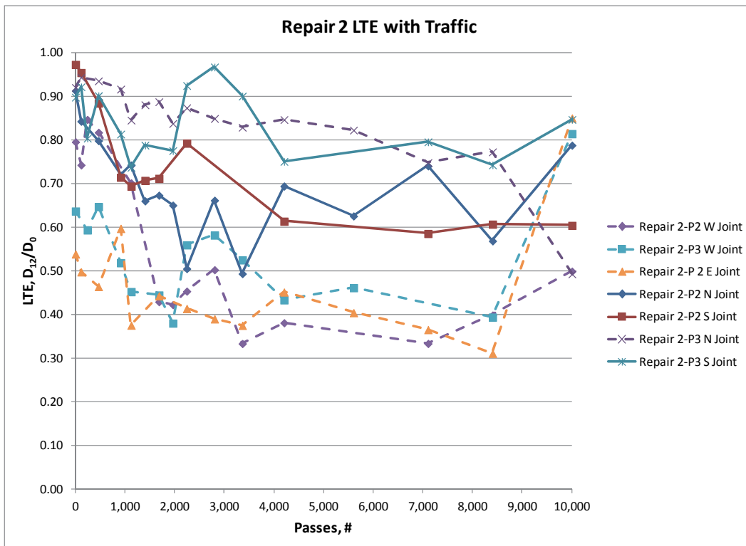
Figure 24. Load transfer efficiency for Repair 2 (Panels 2-3) with traffic.
