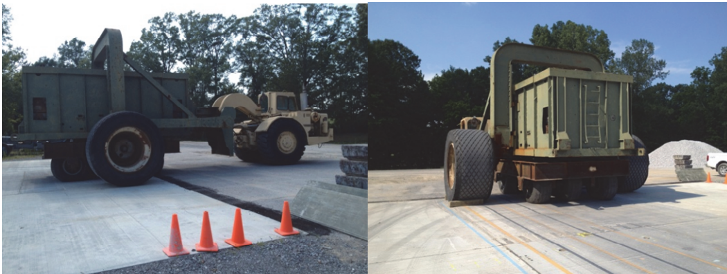
Figure 9. C-17 load cart on test section.
