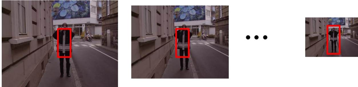
(a) Downsampling the image, size of detection window remains same
