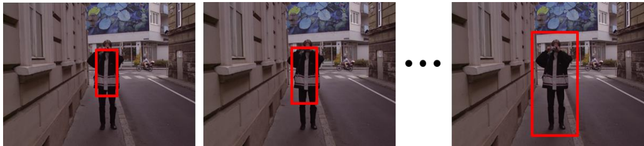
(b) Size of the image remains same, scaling up the size of detection window
