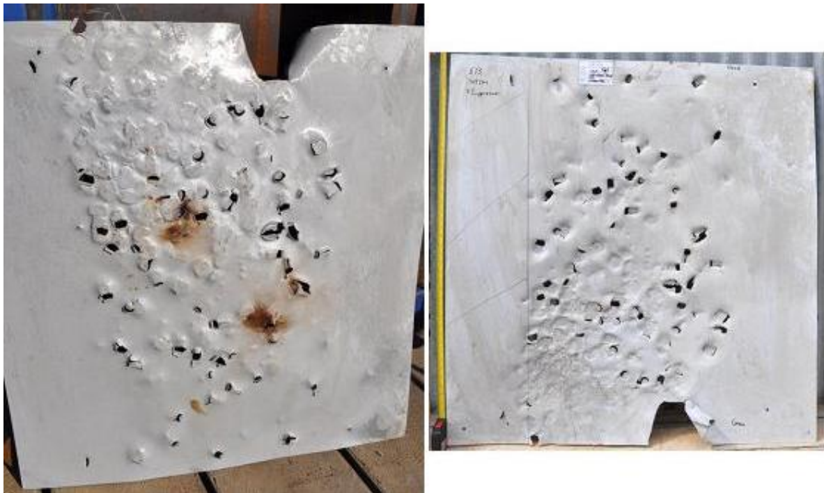
Figure 50: 1 mm thick Al witness plate used to assess ejecta dispersion for a 1xTCM configuration, experiment 13 at a distance of 1014 mm from the top of the propelling charge storage tube. LHS image: witness plate viewed from behind. RHS image: view from front.
