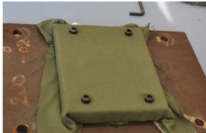
Figure 18: Instrumentation board covered with a cotton and Nomex fabric swatch
