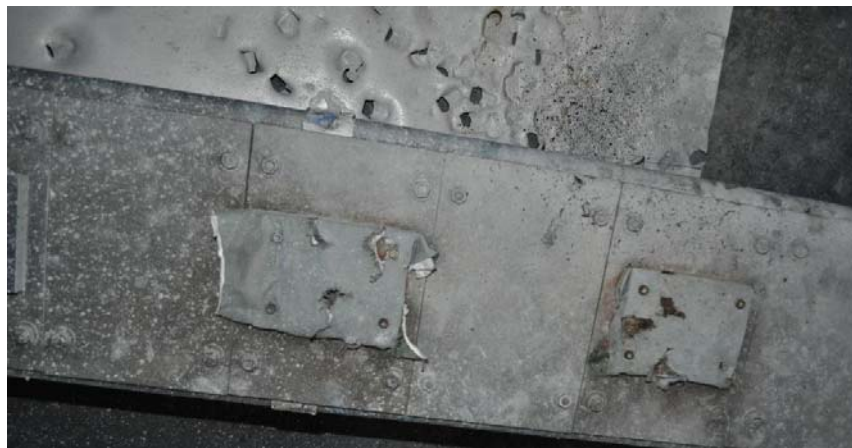
Figure 51: Ejecta damage to Person C in Experiment 13
