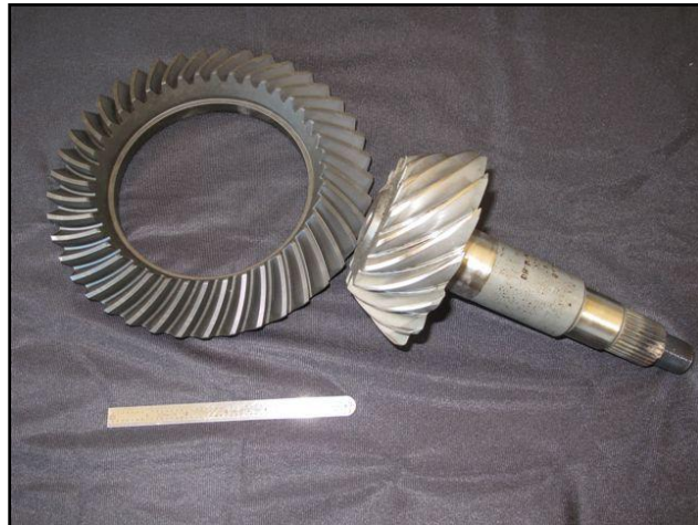
Figure 7. Photograph of the hypoid ring and pinion gears from the M1097A2 rear axle.
