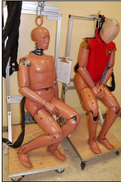
Figure 3. FTSS, Inc., Hybrid III (left) and GESAC, Inc., THOR ATD (right).
