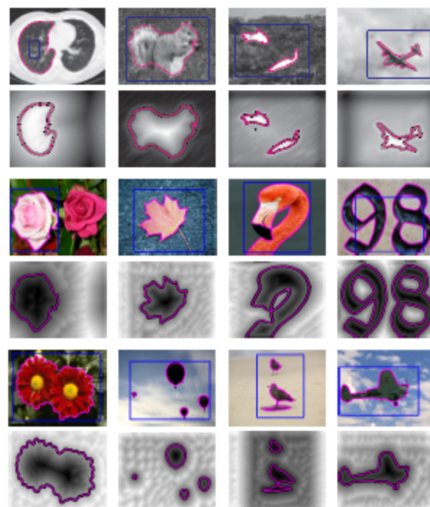
FIGURE 24. Proposed level set-based segmentation method applied to natural images. For each result, we show the segmentation result and the level set function. We plot the initial zero level set in blue, the final contour in pink and the \pm 1, \pm 2 level sets of the final functions in black
