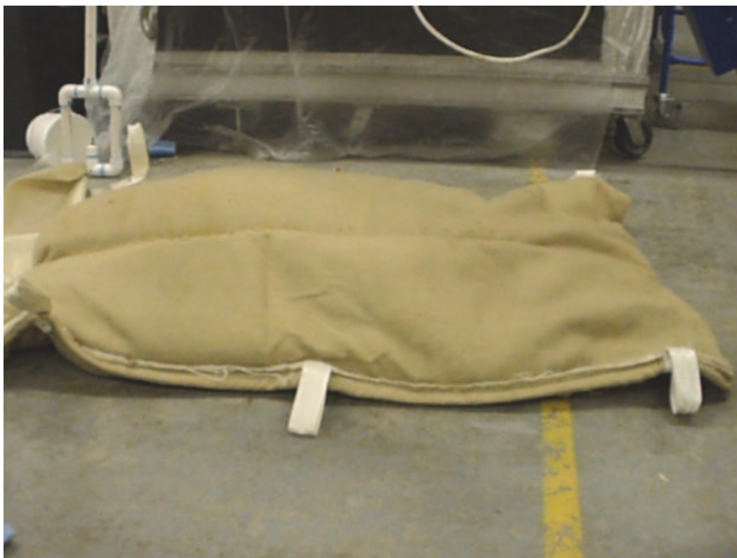
Figure 17. Geobag with internal panels covering horizontal 155 mm M107.
