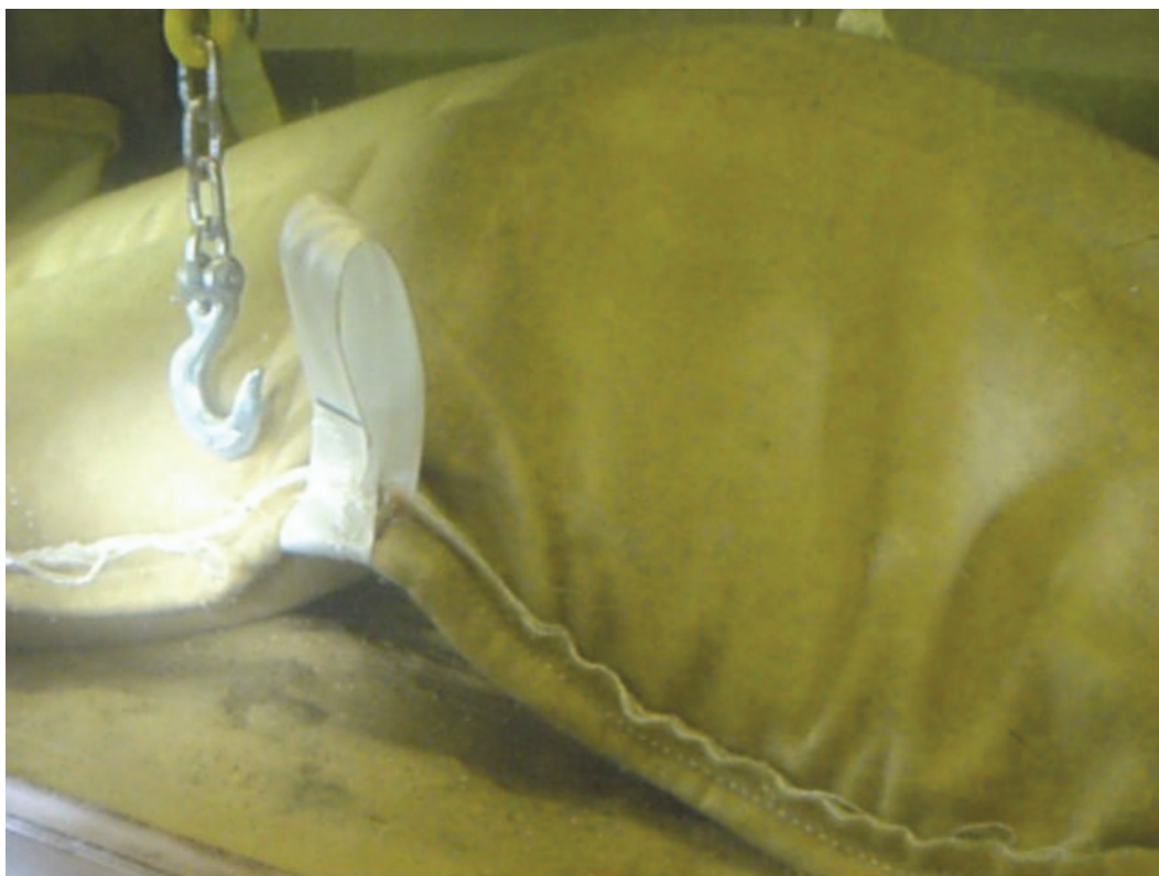
Figure 25. Geobag on inclined 155 mm M107.
