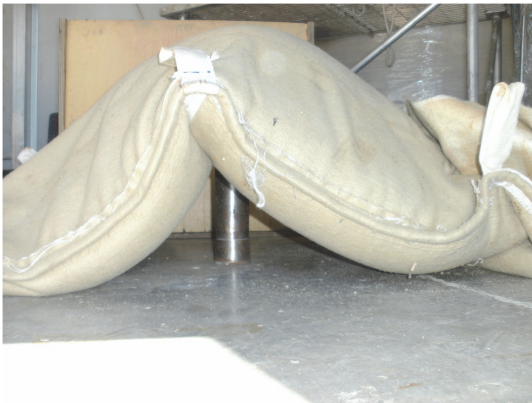
Figure 20. Geobag on upright munition.
