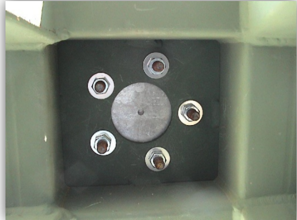
Figure 10. AUMS Host Turret Mounting Pattern
