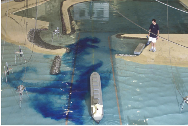
Figure 3. Barbers Point, HI: coastal, fixed-bed, 3D, 1:75 scale model for studying effect of jetties on navigation (Source: Mike Briggs).
