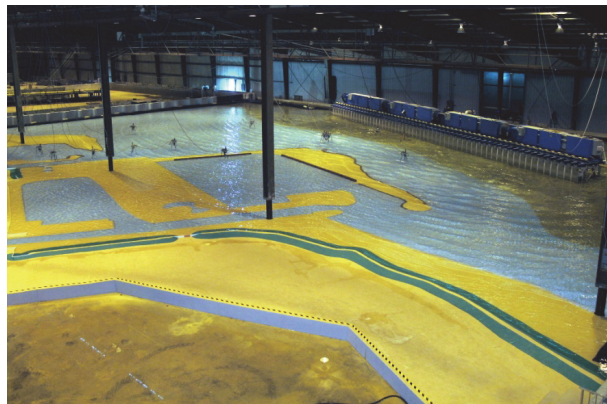
Figure 1. New Orleans 17th Street Canal: coastal, fixed-bed, 3D, site-specific, 1:50 scale model to study flooding and failure of levees due to Hurricane Katrina (Source: Bill Seabergh).
