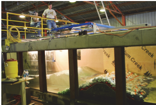
Figure 5. Colorado River: coastal, fixed-bed, 2D model for studying breakwater designs (Source: Don Ward).
