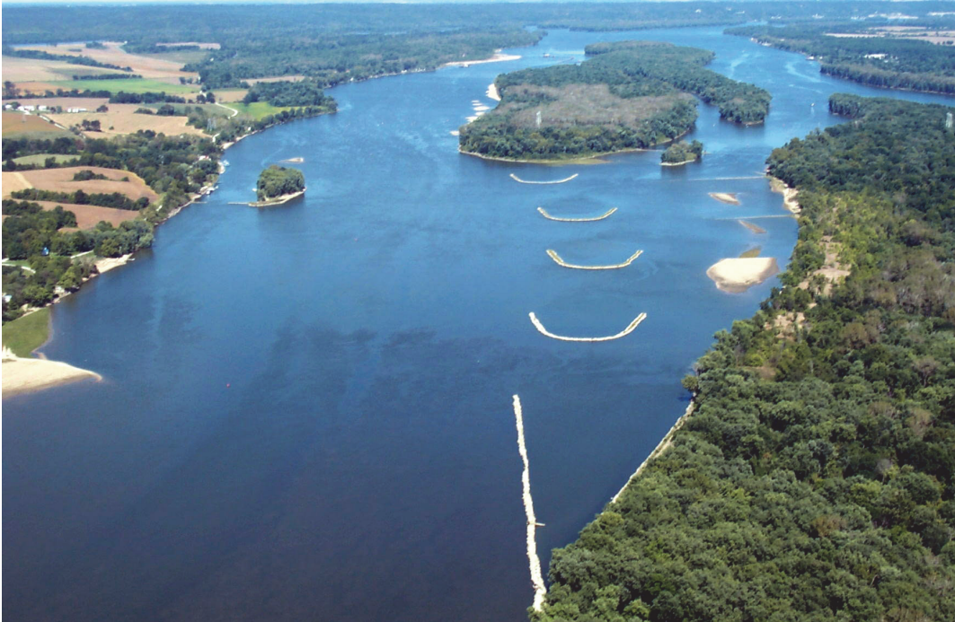
Photo #1. A series of four chevrons along the Mississippi River. Chevrons are horseshoe-shaped structures that both guide river currents to keep the channel navigable and generate low flow pools and small islands immediately down-river, providing habitat for fish and other species.
