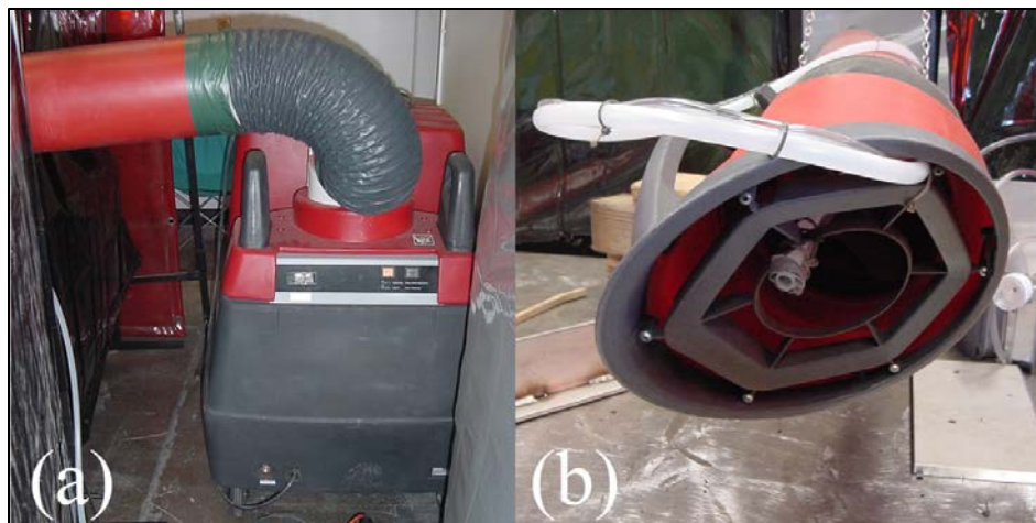
Figure 4. (a) Lincoln LEV collector and (b) sampling inlet on hood face (Photo by Kathleen Paulson)
