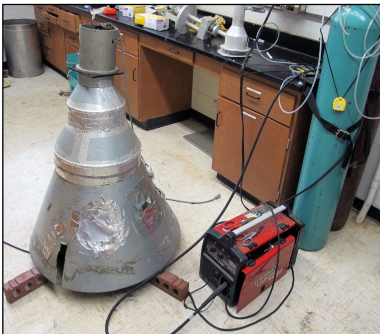
Figure 2. Fume chamber and welding machine (Photo by Jun Wang)
