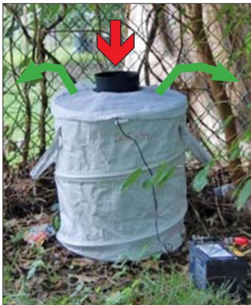
Figure 2. One of the Biogents Sentinel traps placed at each of the 5 positions during the spatial repellent device study. The trap acted as an artificial host for the Ae. albopictus mosquito, using attractant and a 12 volt battery powered system to mimic convection currents created by a human body (green arrows). The mosquitoes enter the trap through the center opening (red arrow) and are trapped for collection.
