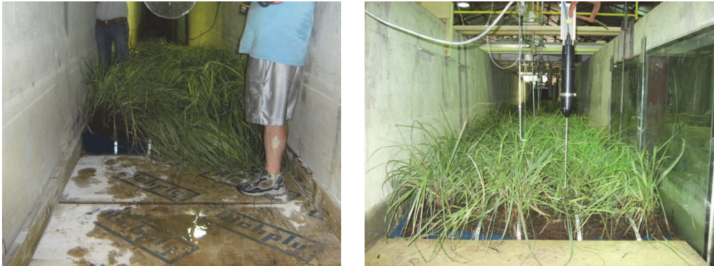
Figure 41. Installing S. alterniflora sections in the flume (left) with completed bed (right).
