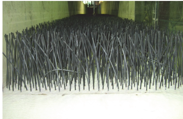
Figure 11. Photograph of artificial vegetation meadow installed in 1.5 m flume ( N = 400 stems/m 2 ).
