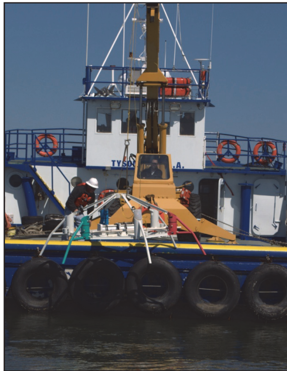
Figure 2-5 Wave gauge and pod being lowered to the seafloor from the Tyson B.
