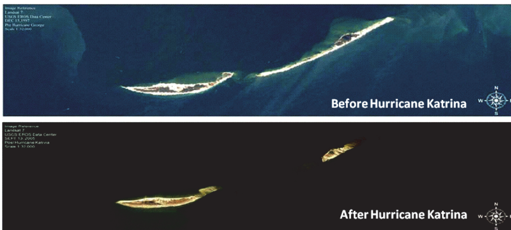
Figure 6-19. Ship Island before (top) and after (below) Hurricane Katrina. Note the significant widening of Camille Cut as a result of Katrina (source: http://soundwaves.usgs.gov/2009/03/ ).
