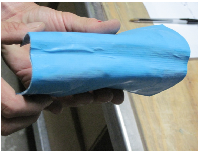
Figure 5. “Bubbling” of drop thread fabric caused by delamination.
