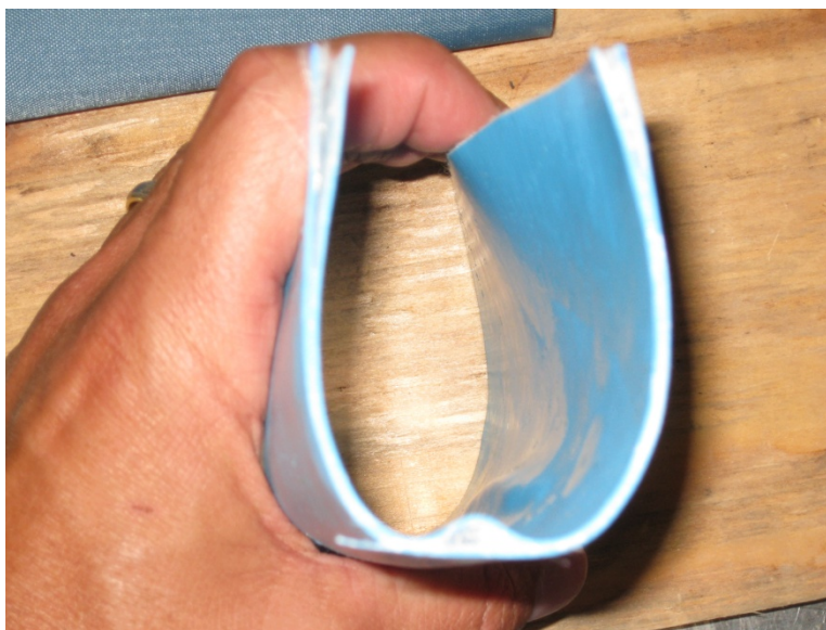
Figure 4. Delamination of drop thread fabric after bending.
