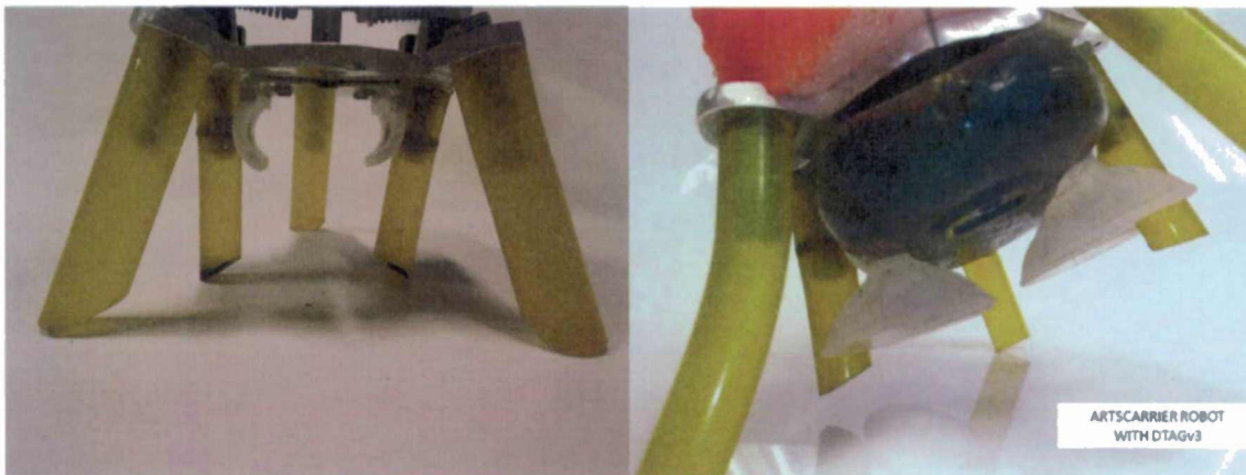
Figure 2: the new ARTSC12 with five GL studs shown with empty docking station (left); and when docking the DTAGv3 (right)
