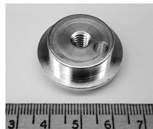
Figure 1. The hand-held signal delay housing. The output side (4.8 mm diameter hole) is shown in this photograph.
