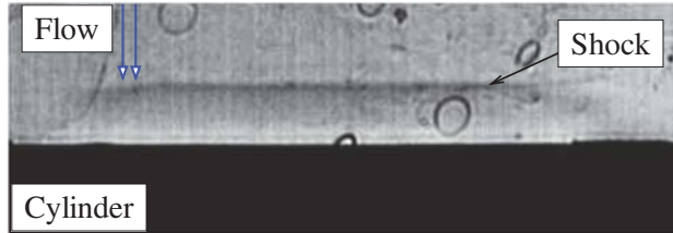
Figure 3. Schlieren image of the bow-shock for Mach 5 air flow over a 6 mm diameter cylinder (top-down view).
