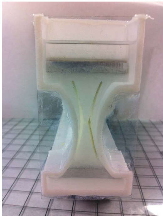
Figure 137. 60 Kcps wet NTG was prepared with 35 hours degassing.
