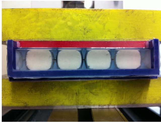
Figure 75. TEES designed and attached short window manifolds on the array. 25K cps silicon oil fluid was used for cyclic test.
