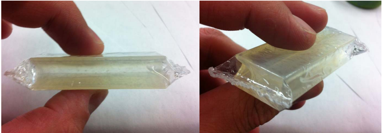
Figure 160. New 13WTGs have no reservoirs and reduced geometrical constraint. Wrapping the cell with polymer film the contained fluids and helped the channel pump.
