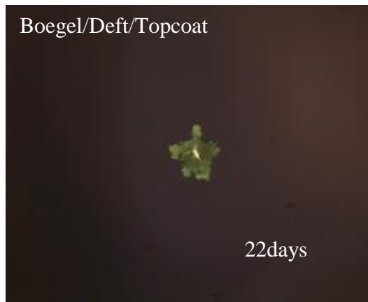
Figure 1.4.15 Images of corrosion sites in Al-Cu thin film at “As deposited” condition under different coating systems exposed to ASTM G85 for different exposure times.
