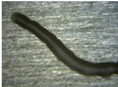
Figure 2.26: Optical picture of active filament growing under PVB after 2 weeks exposure in Kilauea Volcano, HI.
