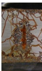
Figure 2.29: Sample photographs of PVB coated steel exposed near Kilauea Volcano for 1 month.
