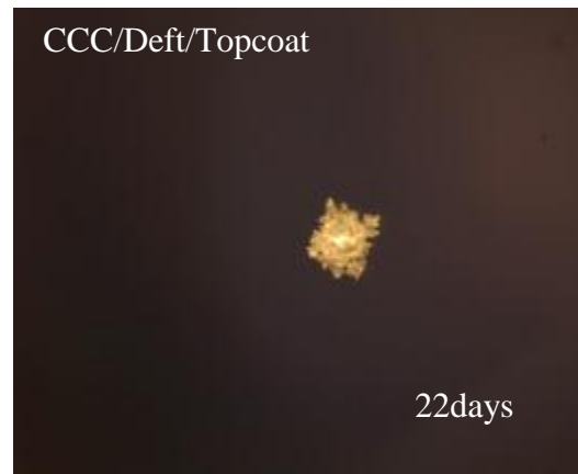
Figure 1.4.15 Images of corrosion sites in Al-Cu thin film at “As deposited” condition under different coating systems exposed to ASTM G85 for different exposure times.
