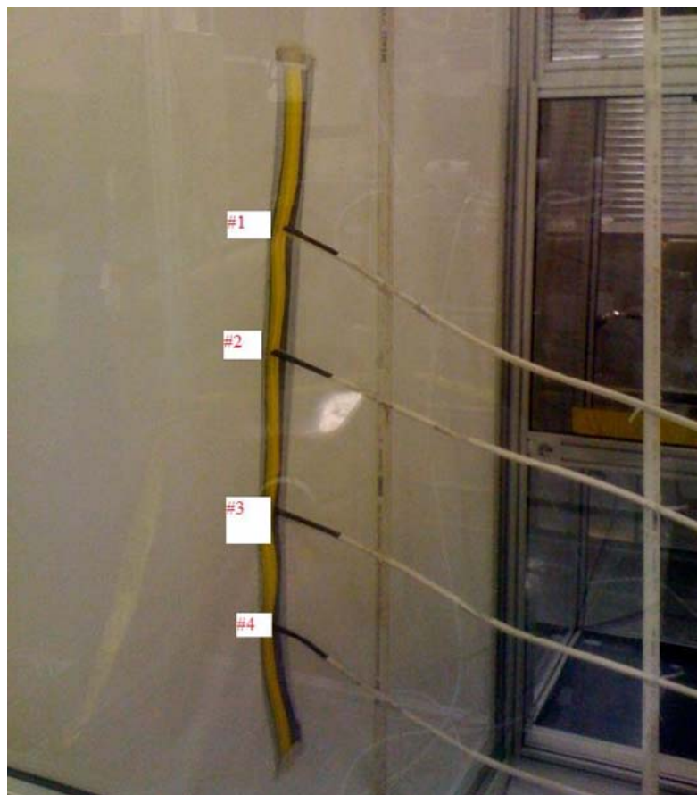
Figure 3. Photograph of sampling line locations in the Toxic Free Area (TFA) compartment; probes were connected to the MINICAMS®.
