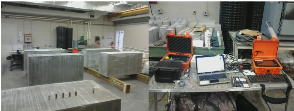
Figure 2: Concrete Test Blocks with Test Equipment in the CFL at NCSU
