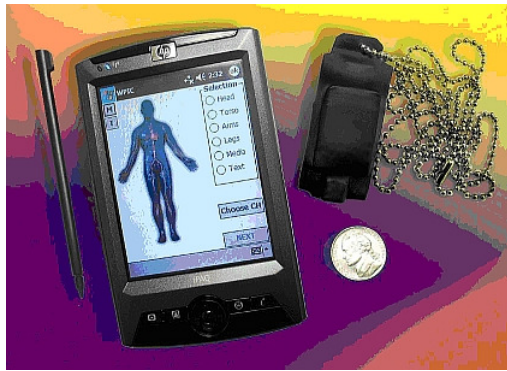
Figure 37 - Electronic Information Carrier (compared in size to AHLTA Mobile on a handheld, and a quarter)
