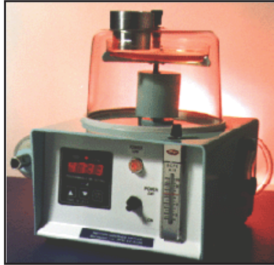
Figure 7. Mattson-Garvin model 220 slit-to-agar (STA) sampler.
