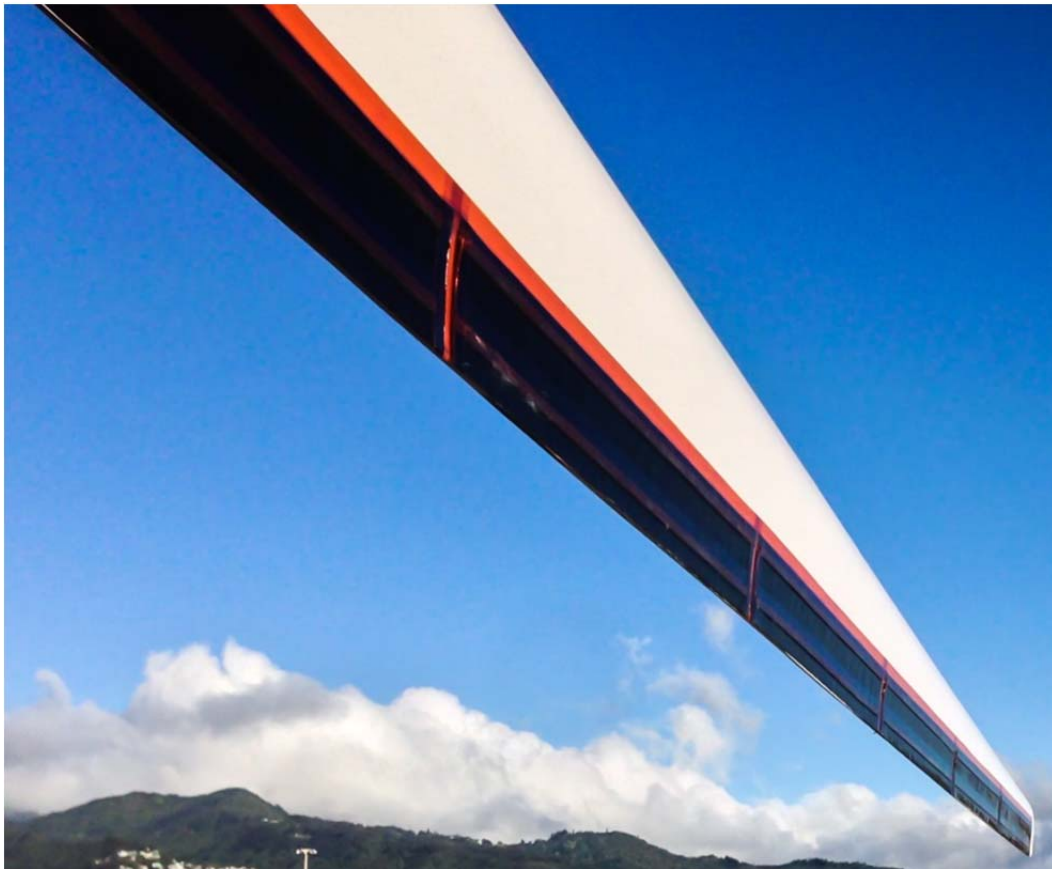
Figure 72. Actuators installed on a VP20 blade. This picture shows the six actuators affixed to one of the three VP20 turbine blades.
