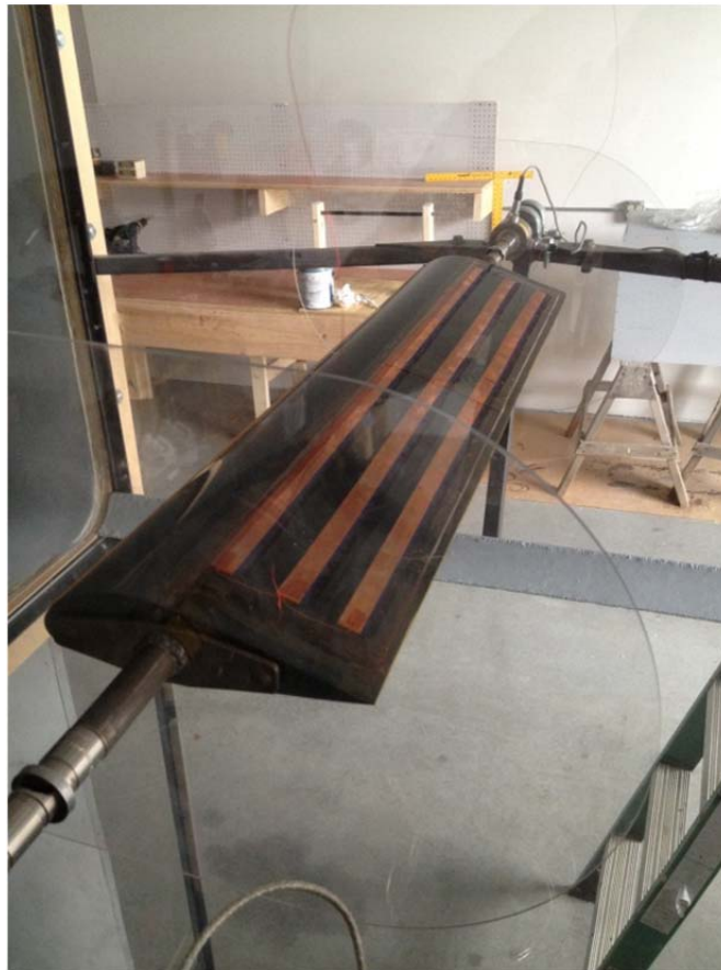
Figure 24. The mid-chord mounted triple actuator. This picture shows the triple 20 mil Cirlex actuator mounted at the mid-chord position.
