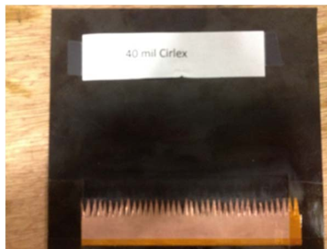
Figure 60. Serrated actuator. This 40-mil thick Cirlex actuator was constructed with a serrated electrode. The serrated electrode provides regions of increased electric field strength, resulting in a measureable increase in thrust. We are interested to know if that increase in thrust comes with a similar increase in gaseous byproducts.
