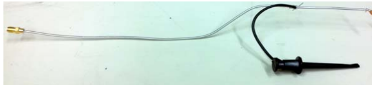
Figure 6: RF probe for the development board. A semi-rigid coaxial line has ground connected to clip and DC blocking capacitor is added. The 50 ohm probe impedance is uncontrolled after the ground clip is added.
