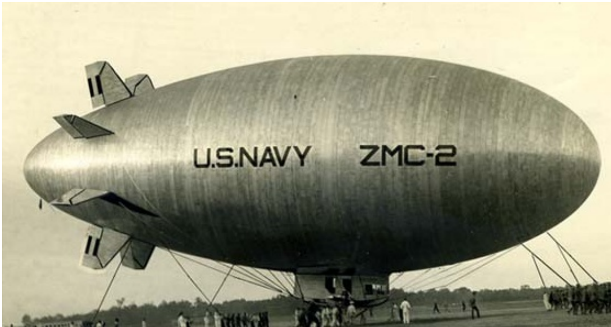
Figure 3: ZMC-2 Metal Clad Airship ca. 1930 [12]
