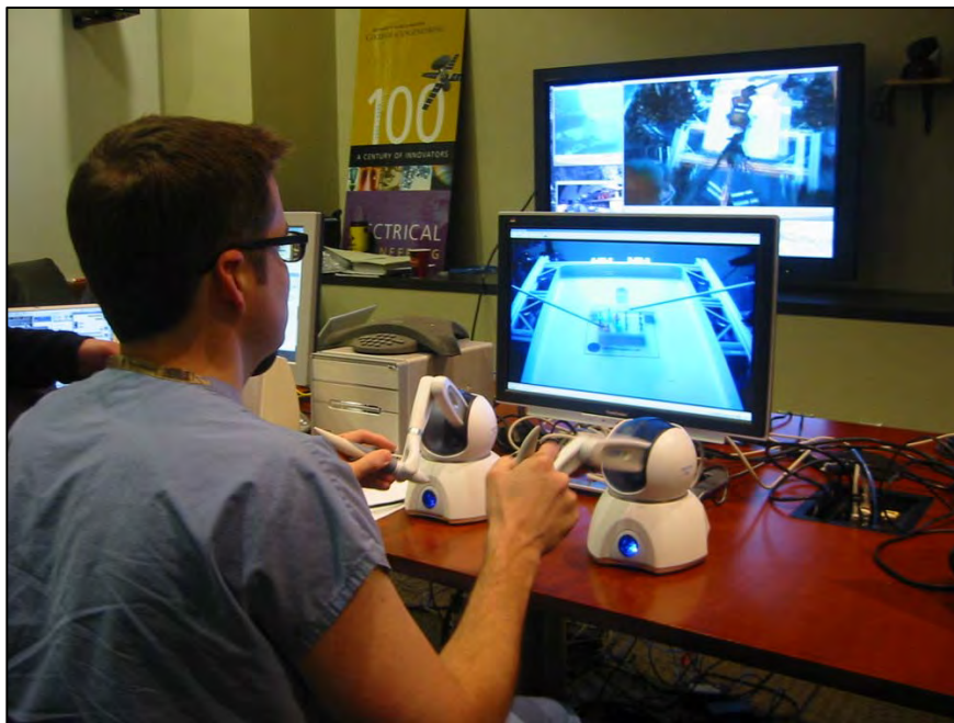
Figure 2. Portable surgical workstation as set up at the NEEMO on-shore site showing Phantom Omni hand control devices and video feed from the underwater habitat.
