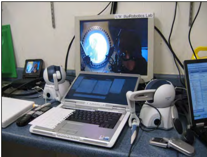
Figure 2. Portable surgical workstation as set up at the NEEMO on-shore site showing Phantom Omni hand control devices and video feed from the underwater habitat.
