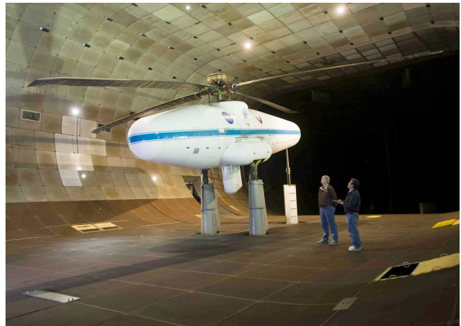
Figure 1. UH-60A Airloads rotor installed in NFAC 40-by 80-Foot Wind Tunnel.
