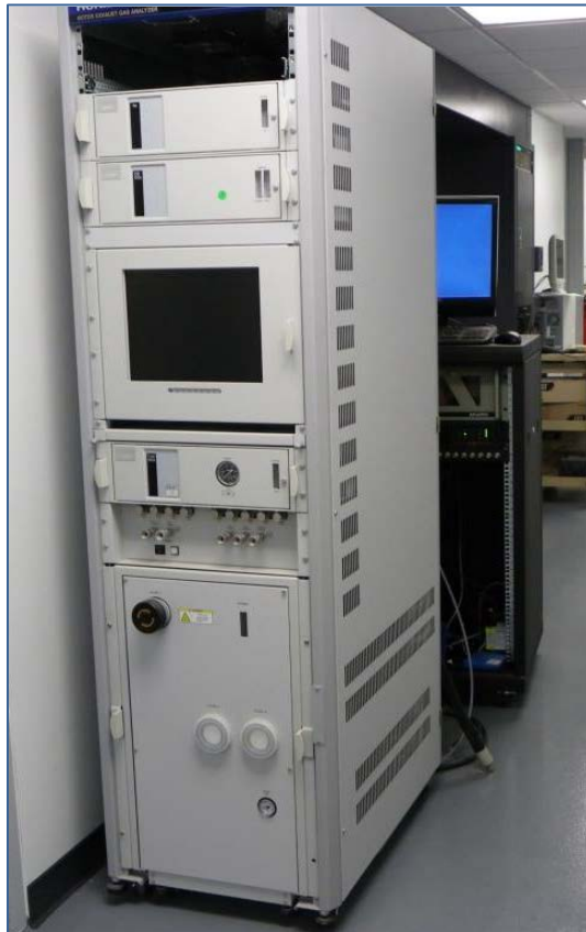
Figure 3. Horiba MEXA 1600D Emissions Bench
