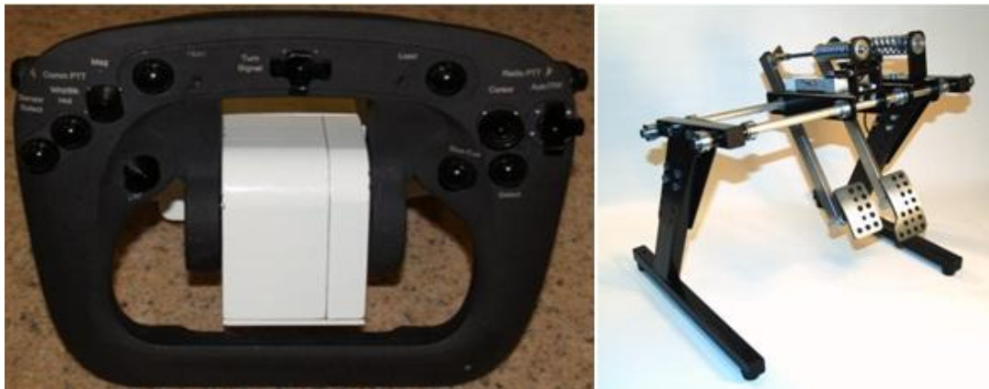
Figure 4: Steering Yoke and driving pedals
