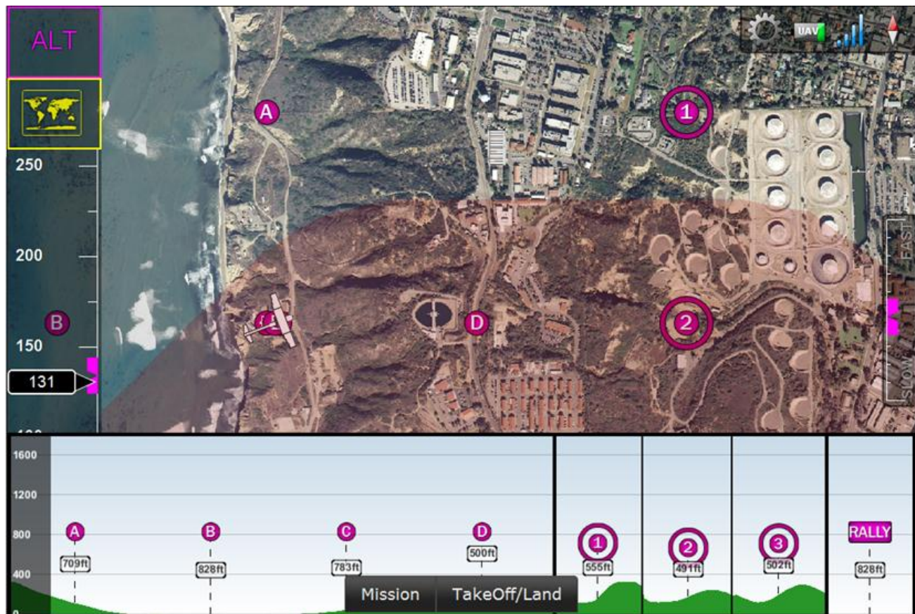
Figure 5. MOCU waypoint altitude mission plans show AGL in the text box while the MSL of the waypoint is shown in the altitude tape on the left.
