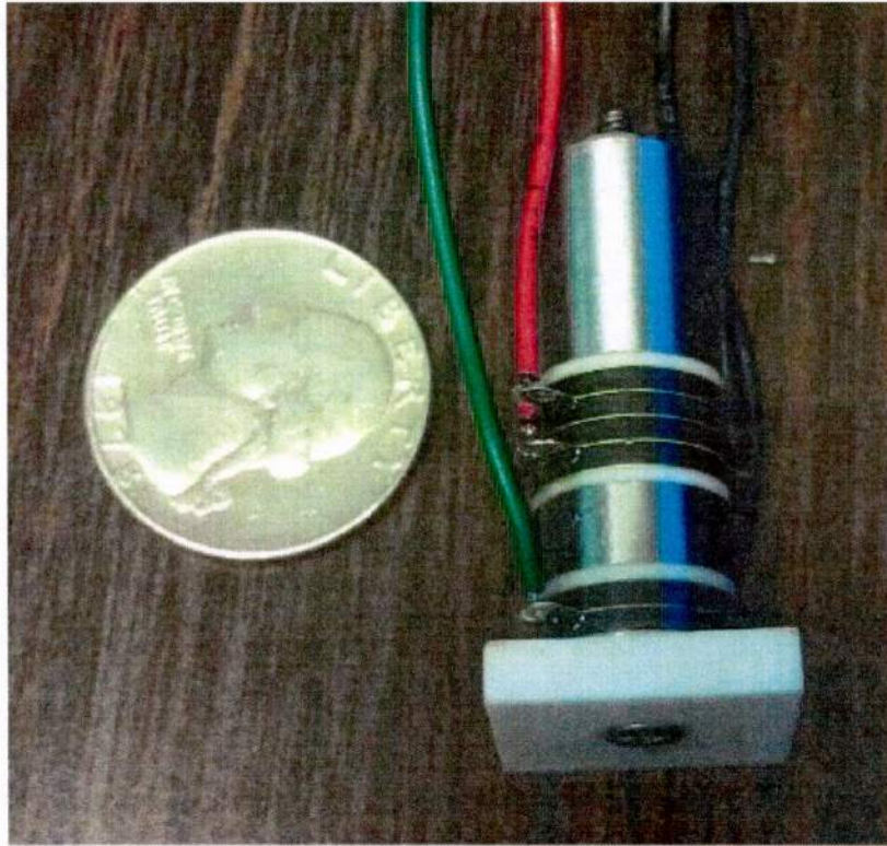
Figure 11 – The first transducer element verified the assembly processes and procedures as verified by electrical bench testing.
