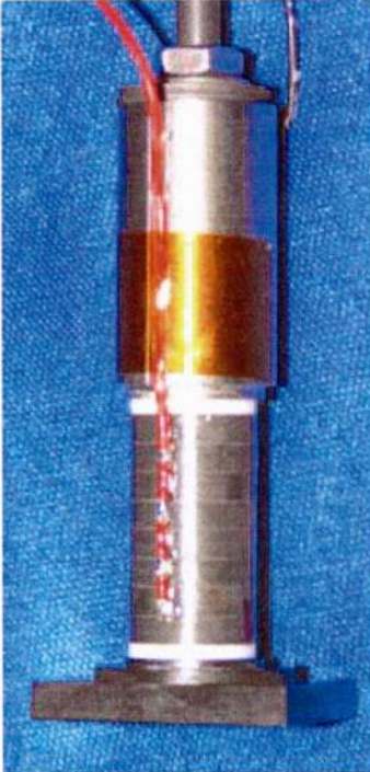
Figure 2 – A singly resonant tonpilz transducer built with PMN-PT single crystal piezoelectric material achieves an octave of bandwidth with high transmitting power factor and an additional half octave of flat transmitting bandwidth having poorer power factor.
