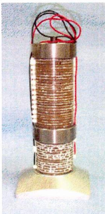
Figure 1 – A doubly resonant transducer element built with PZT ceramic that achieves a bandwidth of approximately one octave. (Figures from reference 1.)
